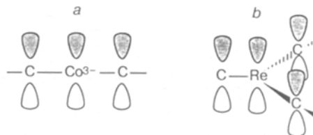
Fig. 2. Role of metal p orbitals in M=C double bonding in the polymeric anions in YCoC and Y_2ReC_2 . a. CoC_{2/2}^{3-} anion in YCoC ; b. ReCC_{2/2}^{6-} in Y_2ReC_2 .
